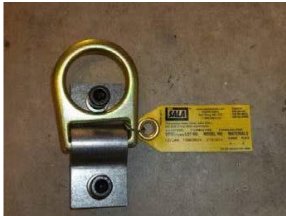
Figure 6 Two-bolt D-ring Anchor Plate attached with 1/2"-13 TPI UNC 1-1/2" long grade 8 socket head cap screws and lock washers (torque to 40 foot-lbs.)
