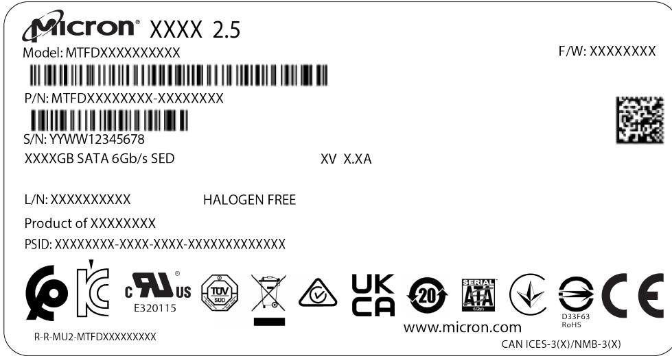
Figure 10: Micron Standard SATA/NVMe 2.5/U.x SSD Label Structures
