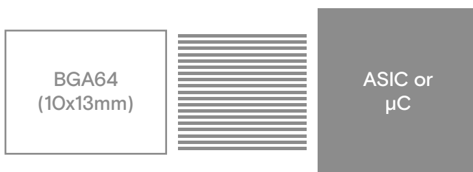
Parallel NOR Flash (50 active pins)
